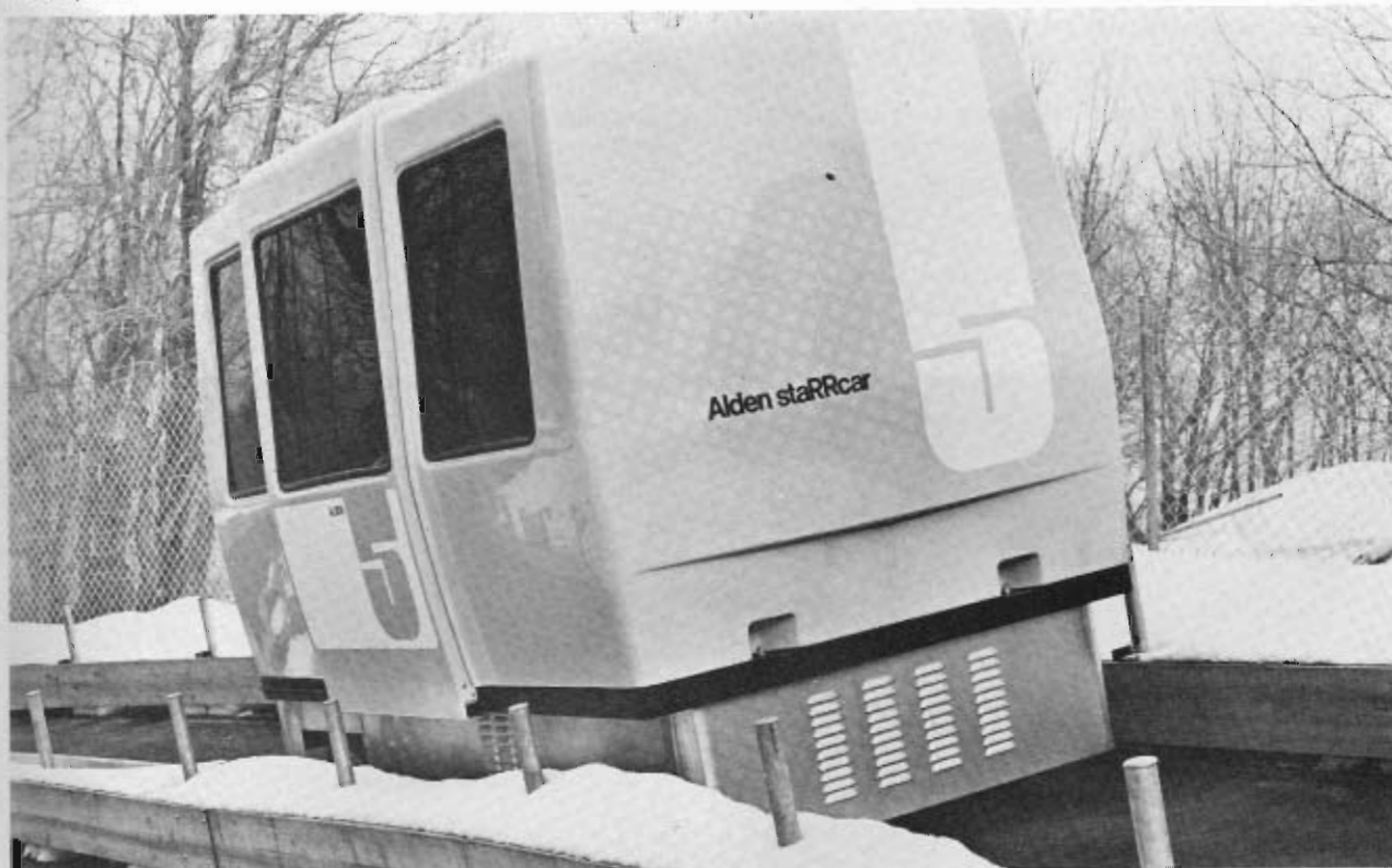
Prototype six-place urban transit system vehicle built by Caldwell for Alden Self-Transit Systems.
